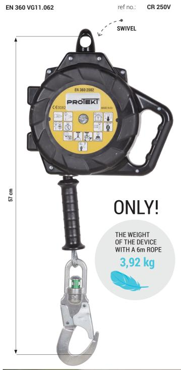
CR 250V self-locking device for vertical operation in a plastic casing with a pull-down steel rope and a swivel mounted in the casing. The device is designed for work requiring significant displacement in relation to the point of attachment. No need to use a shock absorber.
