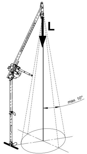
WORKING LOAD "L" CAN BE DIRECTED VERTICALLY ONLY (TOLERANCE ±10°).
