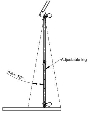
ADJUSTABLE LEG MUST ALWAYS BE PERPENDICULAR TO THE GROUND (TOLERANCE  $\pm$  10 °).
