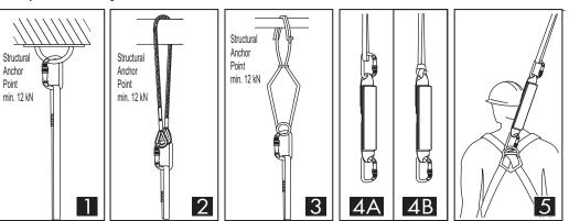
NOTICE: - In determining the space under the workplace required to arrest the fall, consider the sling as an additional element that extends the distance for arresting a fall
