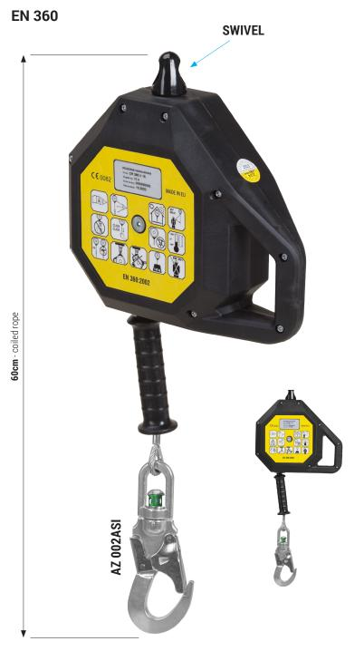
CR 260V self-retracting fall arrester with unrolled steel rope in a casing made of plastic, equipped with a swivel. It has a comfortable side handle. The rope is made of galvanized steel with a diameter of 4 mm. The device is designed for work requiring significant displacement in relation to the attachment point. No need for a safety shock absorber
